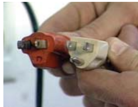
Cords without ground plugs expose individuals to becoming the ground path for electricity.
