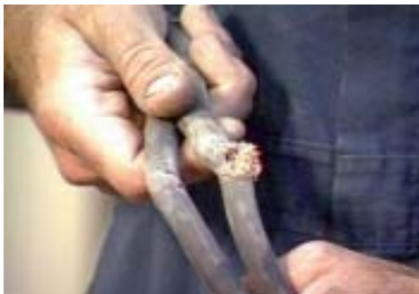
A damaged cable is a serious electrical hazard.
