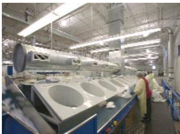
Top: Employees at the COMTEX health care laundry facility in Columbus, Ohio, use chutes to sort soiled laundry into the proper categories.
