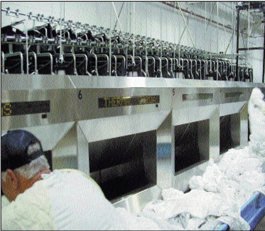
Automated counting/sorting systems, like this one from E-Tech, Minneapolis, increase unloading speed, reduce labor, set standards for unloading trucks, and improve accuracy.
